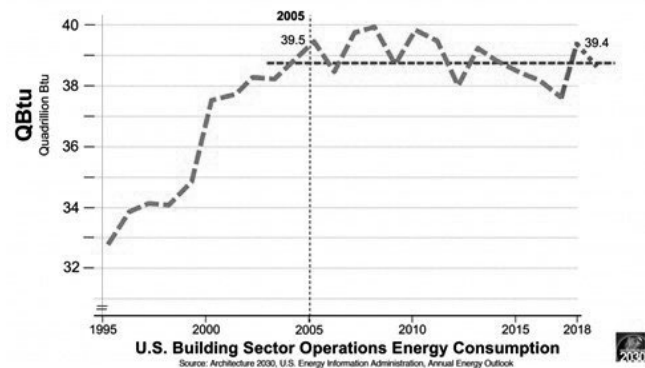
Figure 1. No increase in operational energy consumption since 2005 despite ongoing construction of new buildings. Source: Architecture 2030, accessed January 2020.
